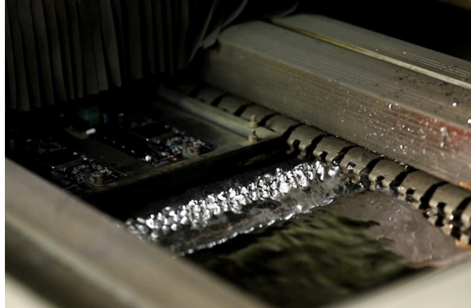
Boards in a fixture approaching the solder wave in a wave soldering machine
